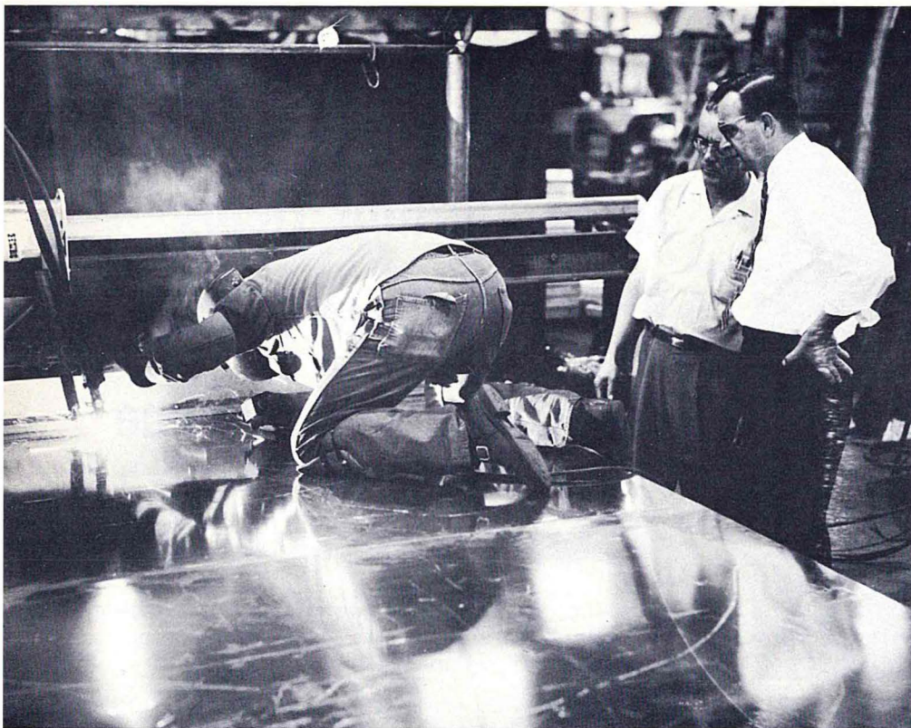
Welding Engineer John Vasin and Foreman Marv Powell watch the automatic seam welder as it works on an aluminum assembly unit.
